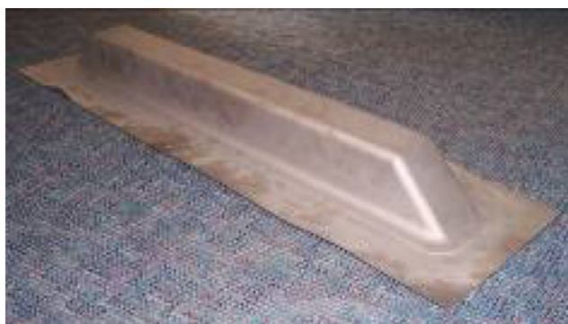
Fig. 6 Actual SPF part formed for comparison to numerical models
